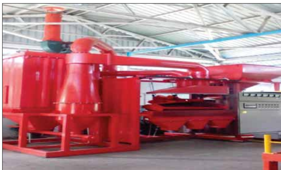
Figure 1 : Air Fluidized Vibrating Deck Separator setup
