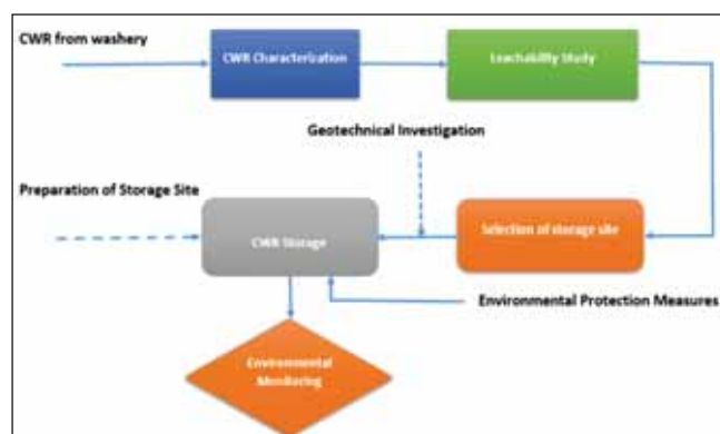
Diagram 1 : Schematic diagram of technical SOP for storage of CWR on surface
